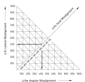
Prior to installation, the shaft misalignment must be measured. Each type of misalignment (axial / lateral / angular) must be calculated and checked against this chart.
