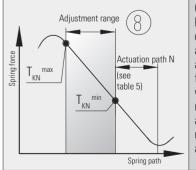
**Caution:** R+W torque limiters have disc springs with a special characteristic. The torque adjustment range lies within a specific range of positions for the disc spring, outside of which the torque limiter can not function. It is important to always stay within the min.max. of the specified torque adjustment range.
