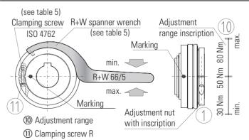
R+W torque limiters are preset and marked with the desired disengagement torque setting at the factory. The min. and max. of the torque adjustment range (10) are also marked on the adjustment nut (1). The disengagement torque is continuously adjustable within the prest range (10) by turning the adjustment nut, increasing or descreasing the tension on the disc springs (2).
